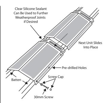
Each unit can be carefully cut/shaped/notched according to roofscape. Hip and Ridge ends should be finished with the appropriate end cap.
