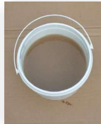
Once catalysed the resin turns orange/brown
