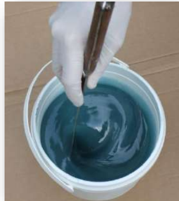
Mix thoroughly to ensure all resin is catalysed
