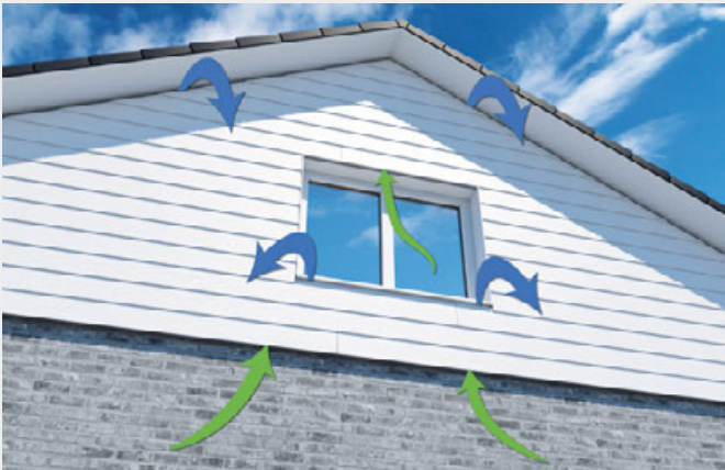
→ Green: Air inlets → Blue: Air Outlets
