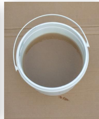
Once catalysed the resin turns orange/brown
