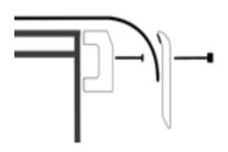
• Fix the 25mm x 40mm back plate to the fascia at the edge of the roof.
