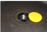
2) Remove the circular section of membrane and the yellow protective cap from the outlet.
