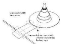
Apply ClassicBond uncured T-Joint Patches where pipe seal intersects a field splice.
