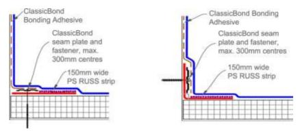
All unreinforced EPDM's and most other single ply membranes produced, regardless of manufacturer, require mechanical securement to eliminate shrinkage and to install in accordance with manufacturers specifications.
